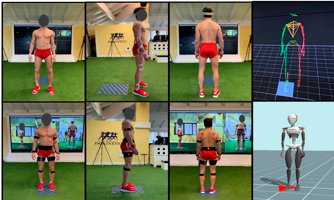
Figure A1. Motion capture systems used in the study: (top row) Plug-in-Gait VICON marker-based protocol in (from left to right) front, side, back, and 3D-environment view; (bottom row) Full Body Xsens inertial sensors protocol in (from left to right) front, side, back, and 3D-environment view.
