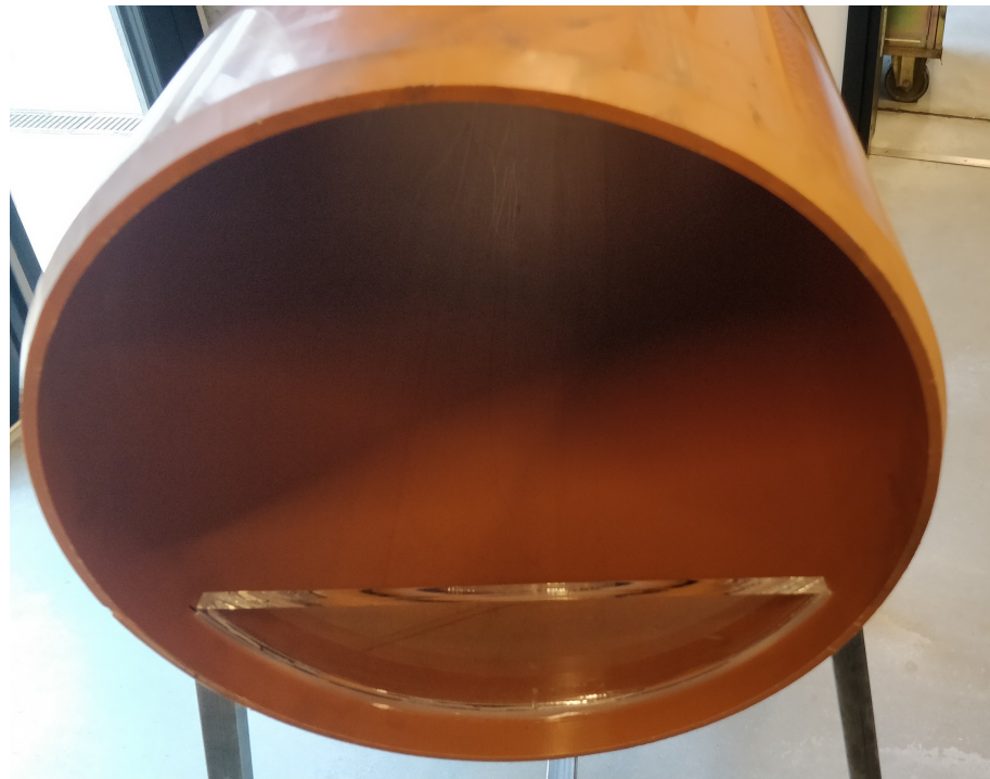
Figure 8. Water level setup. A piece of acrylic glass is inserted at both ends of the pipe in order to accommodate water.
