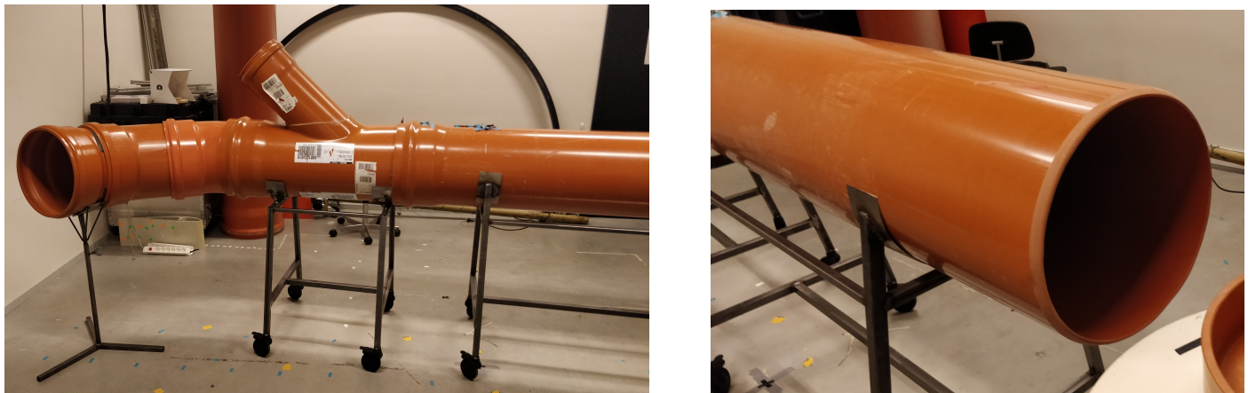
(a) View of the bigger setup consisting of a single branch pipe and bends.
