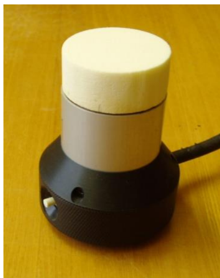
Figure 1. OSA sensor and a PUR foams' sample.
