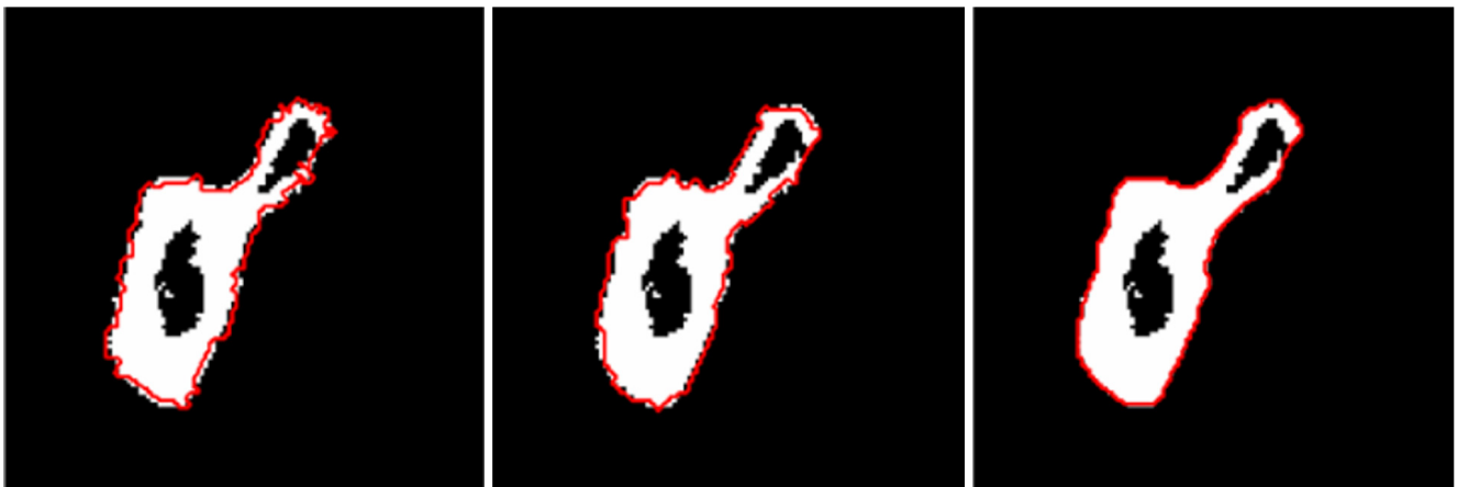
Figure 5 Snake curve convergence results for different parameters, with the weight coefficient of internal force terms gradually increasing from left to right.
