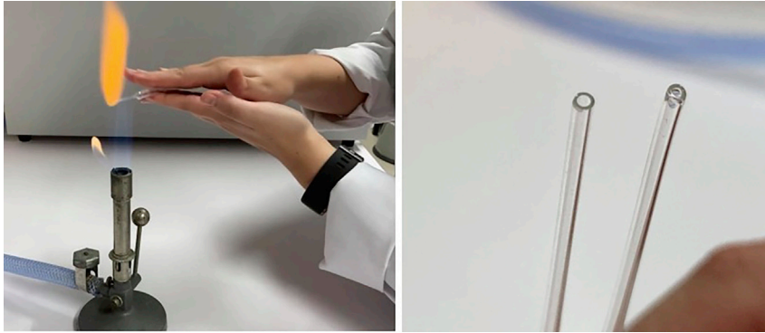
Figure 2. Fire-polishing of the glass Pasteur pipet
