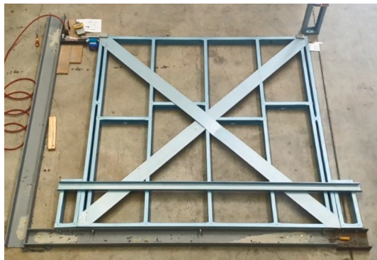
Fig. 16. Tested frame with 150 mm strap bracing [72].
