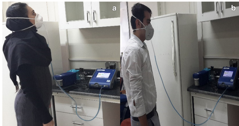
Fig. 1 The participant while performing the QNFT procedure using the PortaCount® fit tester model 8038
