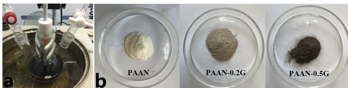
Figure 16. (a) Picture of the polymerization process and (b) the obtained powder sample.
