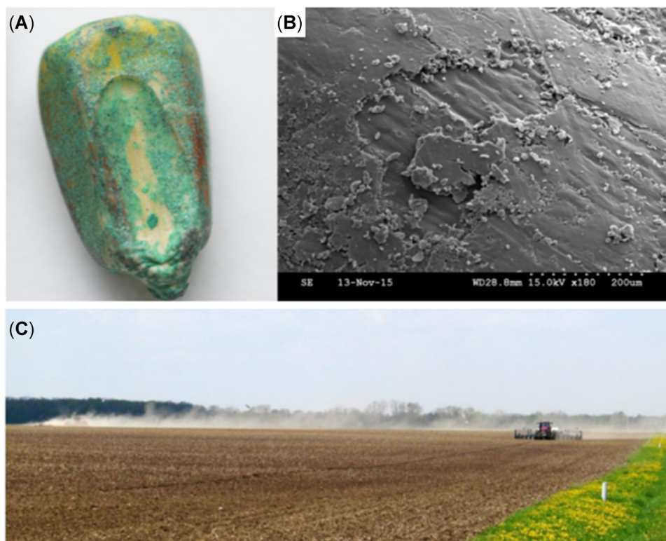
FIGURE 1: Seed treatments are applied to seeds as flowable solids that dry to form a coating. In corn, this coating results in visibly patchy coverage of the seed (A). The seed treatment forms particles of varying size on the surface of the seed as captured using scanning electron microscopy (SEM), (B). The striated surface visible in the center of the micrograph is the seed surface. Particles of the seed treatment coating are then emitted as planter dust during the sowing process (C). Macrophotography was performed by M. Spring and SEM preparation by K. Kaszas.
