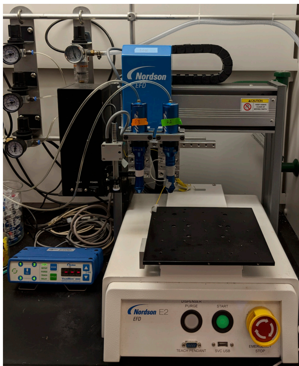
Figure 2. Customized fluid dispensing robot system (Nordson EFD) capable of extrusion-based 3D printing with two print heads.
