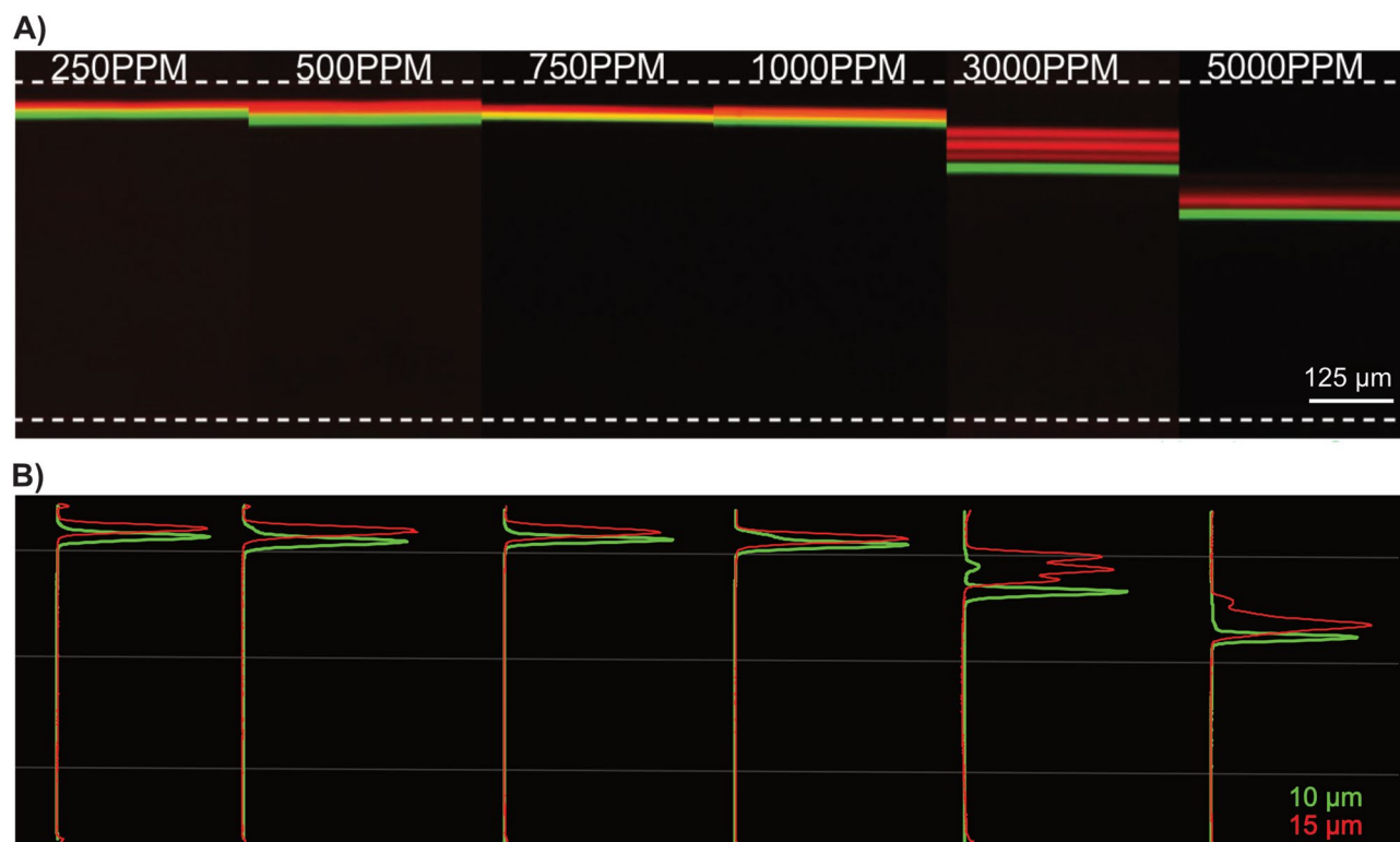
Figure 4. Particle equilibrium focusing position at different PEO concentrations. (A) Fluorescence image of 10 (green) and 15 \mu\text{m} (red) particles at the 10th turn for different PEO concentrations. The particle focusing position is pushed away from the outer wall, especially for 3000 PPM and 5000 PPM. Scale bar: 125 \mu\text{m} . (B) Corresponding overlapped cross-sectional intensity of the 10 and 15 \mu\text{m} particles.
