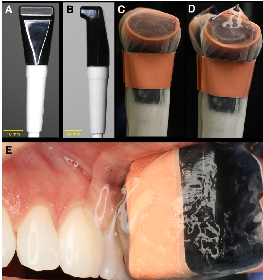
Figure 1. Miniature-sized probe prototype (L25-8). A) Frontal view. B) Lateral view. C) Frontal view of the probe after its preparation for clinical use. D) Ultrasound gel applied on the probe. E) Clinical picture showing the application of the ultrasound probe at the midfacial aspect of an implant site (left central incisor).
