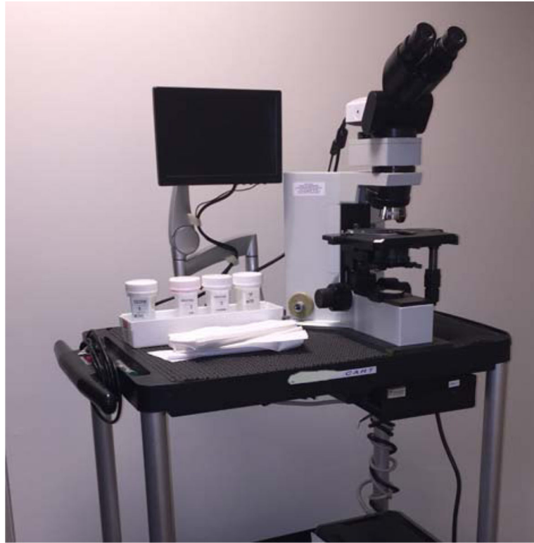
FIGURE 1. RMT® equipment used for telecytology with live image transmission installed in a mobile cart
