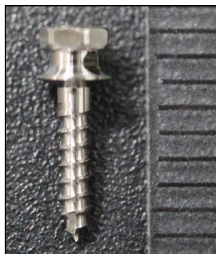
Figure 1. An image of Ti6Al4V miniscrew. Thirty miniscrews (Jeil Medical Corporation, Seoul, South Korea) that were 1.3 mm in diameter and 6 mm in length were used in miniscrew insertion tests. 1 scale = 1 mm.
