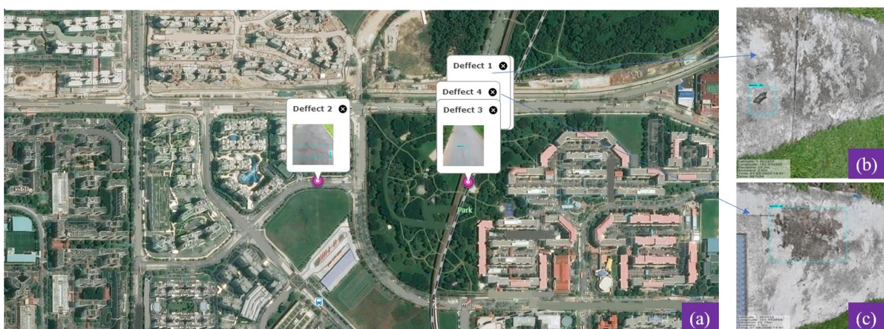
Figure 8. Independent trial for the mobile mapping system and the defect identification. (a) Defect location on global map, (b,c) detected defects and patches.
