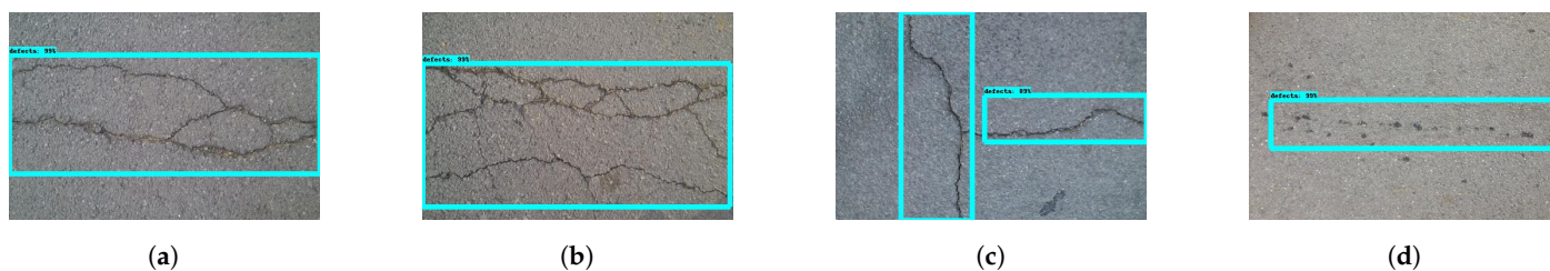
Figure 16. Defect detection results for CrackForest dataset in (a–d).
