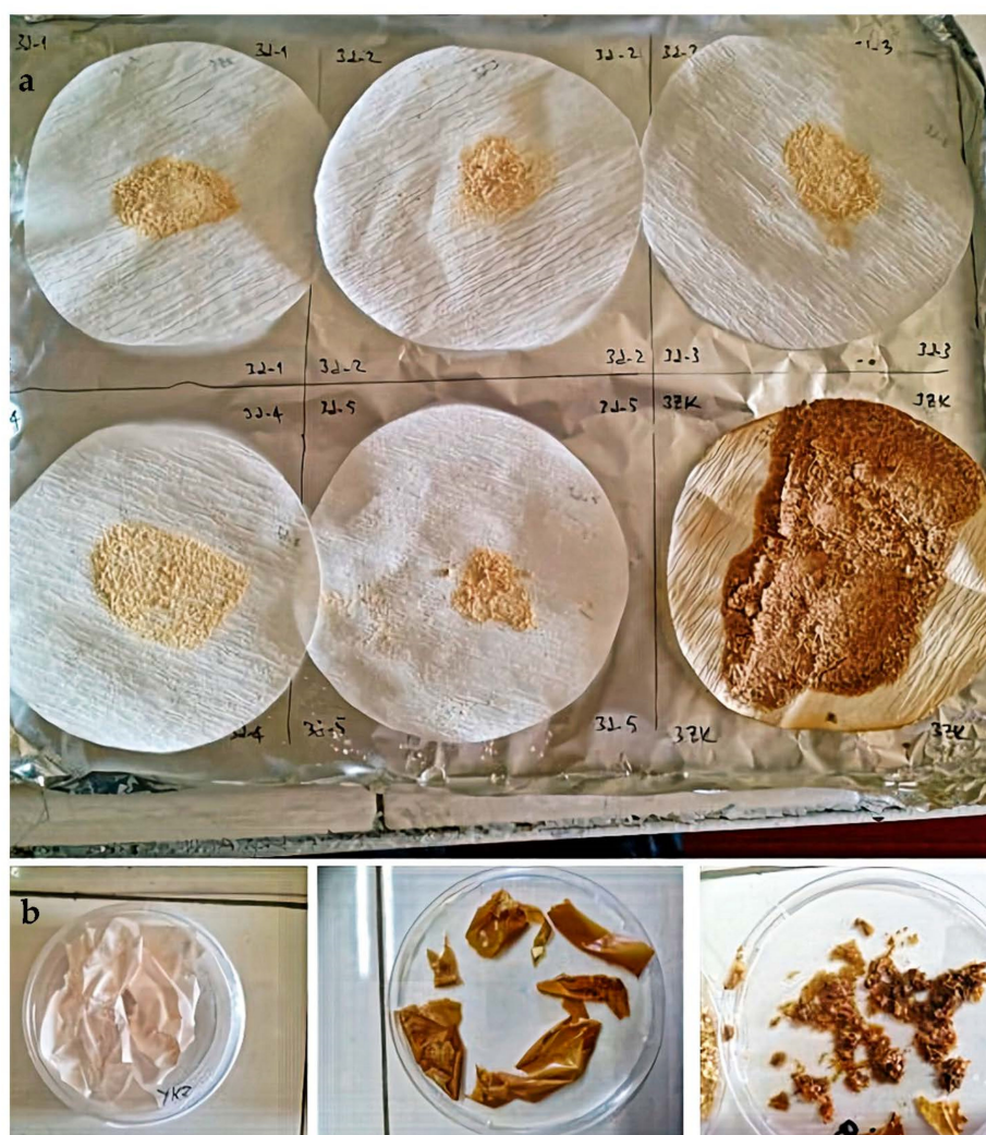
Figure 9. Images of eggshell membrane (a) from foam separation process; (b) before and after OLE adsorption in a batch experiment.
