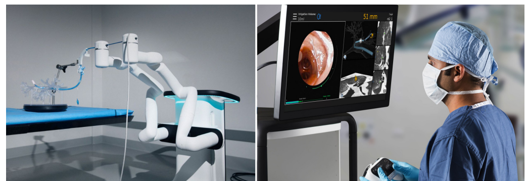
Figure 1. The Monarch robotic endoscopy platform (Auris Health Inc., Redwood City, CA, USA), as an example of image-guided surgery device.
