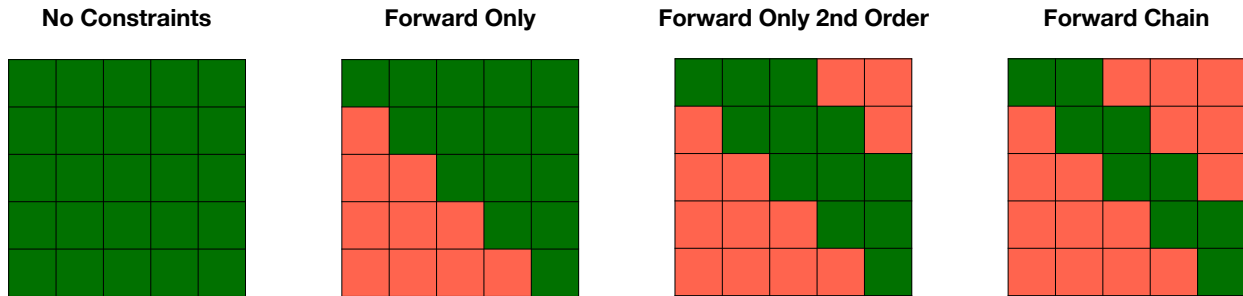
Figure 1: The types of constraints that can be set on transition probabilities of Hidden Markov Models (HMMs). Each constraint is represented as a K \times K matrix, where K is the number of states. The four examples illustrate constraints as green (possible route between states) and red (restricted route between states).
