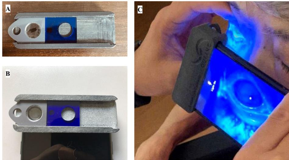
**Figure 1. Characteristics of the Smart Eye Camera (SEC) invented for the evaluation of dry eye disease.** (A) The hardware, which contains the basal component which fits into the iPhone 7. The blue filter fits above the light source, and a convex macro lens is placed above the camera. (B) The SEC equipped to the iPhone 7. (C) The recording interfaces.
