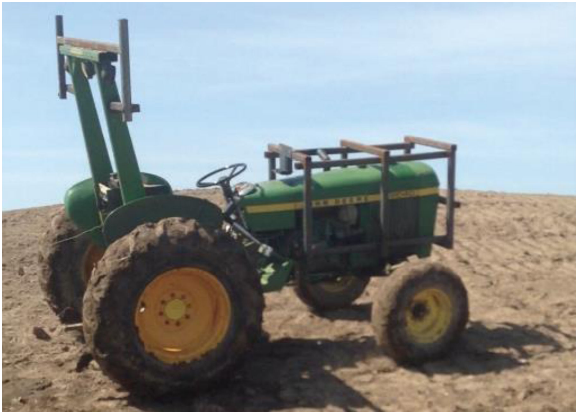
Figure 7. Modified remote-controlled John Deere 2040 2WD tractor
