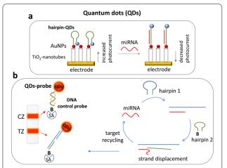
**Fig. 4** a A photoelectrochemical sensing system based on a decrease in the signal, as quantum dots (QDs) are moving away from the electrode's surface upon hybridization of target miRNA to DNA hairpin/AuNPs/TiO<sub>2</sub>NPs-decorated fluorine-tin oxide electrodes. **b** A lateral flow assay based on QDs-DNA as reporters and SDA target amplification for miRNA detection. *AuNPs* gold nanoparticles, *TZ* test zone, *CZ* control zone, *SA* streptavidin, *B* biotin
