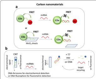
**Fig. 3** a Fluorescent carbon dots (CDs) coupled to a DNA probe are quenched by gold nanoparticles (Au) or MnO<sub>2</sub> nanosheets, phenomenon that is then hindered by hybridization of miRNA target. **b** DNA-carbon nanotubes with T7 exonuclease-assisted or DSN-assisted target recycling were used for the electrochemical or fluorometric detection of miRNA. *CNT* carbon nanotube, *exo* exonuclease, *FRET* fluorescence energy transfer, *DSN* duplex-specific nuclease
