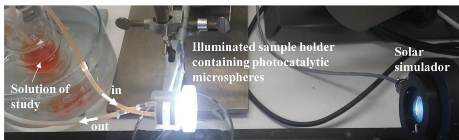
Figure 2. Photograph of the experimental set-up (continuous flow) used for the photocatalytic tests.
