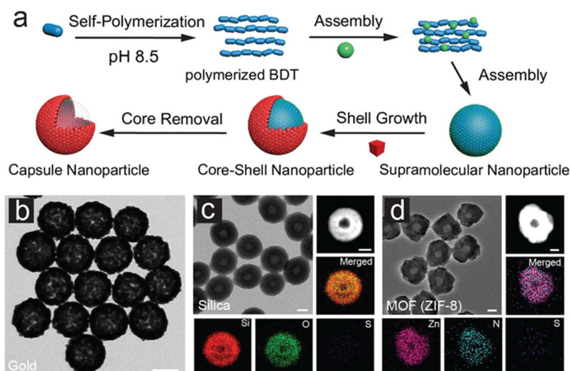
Fig. 17. (a) Synthetic strategy for particle engineering using pBDT–TA supramolecular networks. The polyphenol-stabilized particles subsequently allow for the growth of diverse shell materials on the particles. TEM images of (b) Au (c) silica, and (d) MOF hollow structures after removal of the pBDT–TA core. Insets in image (c) and (d): HAADF-STEM images of representative silica and MOF hollow particles and their corresponding EDX mapping results. Reproduced with permission. Copyright 2020, Nature Publishing Group.
