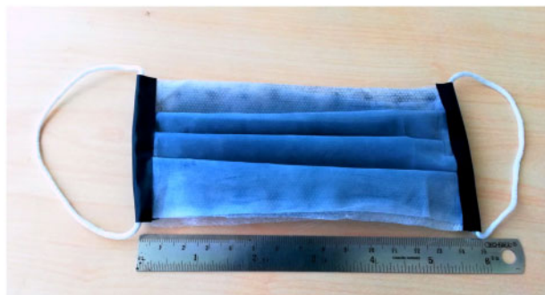
Figure 6: Photograph of the rechargeable PPDFGO tri mask where the three layers are simply stitched together.
