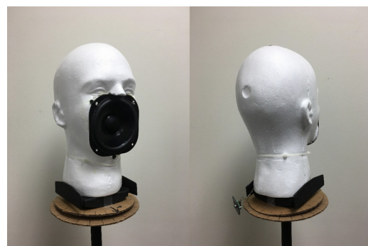
FIG. 2. (Color online) White noise was presented through a head-shaped, custom mouth simulator: (1) with a “listener” microphone placed at distances of 3 and 6 ft to measure acoustic attenuation relative to the no mask condition, and (2) while rotating it in 15 degree increments with the “listener” microphone placed at a fixed distance of 6 ft.
