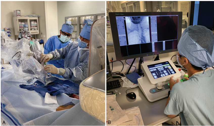
FIG 1. A, Sterile Corpath GRX patient-side robotic system during setup. B, Lead-shielded remote Corpath GRX control station during cerebral angiography procedure.
