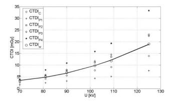
**Fig 3.** CTDI values for center, periphery, and the calculated CTDI<sub>w</sub>. The solid line represents a quadratic fit for the CTDI<sub>w</sub> which was used for subsequent calculations. The correlation coefficient amounted to R = 0.98.
