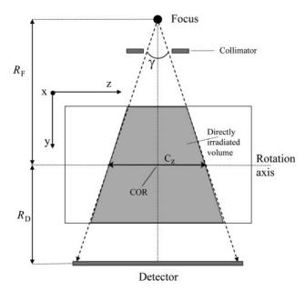
**Fig 2.** Geometry definitions for the y/z plane COR is the center of rotation,  $C_z$  is the beam width at the COR (ie, collimation), and  $\gamma$  is the cone angle.  $R_F$  is the distance from the focal spot to the COR, and  $R_D$  is the distance from the detector to the COR.
