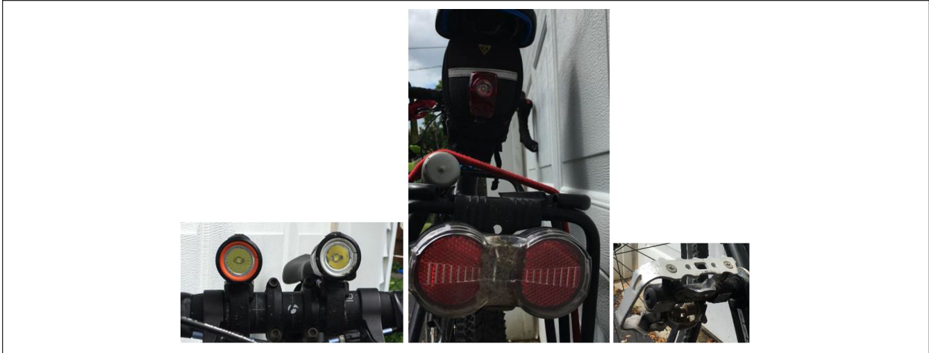
Figure 1. Illustration of redundancy on a bicycle: (a) two headlights, (b) two taillights, and (c) two-sided pedals (one platform, the other “clipless”).
