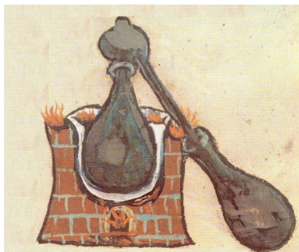
Figure 4. An ancient distillation apparatus—alembic (lat. alembicus ); scheme of an alembic from a medieval manuscript [35] (modified).
