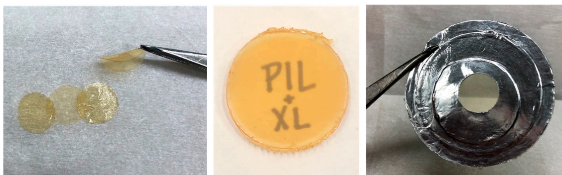
Figure 3. Transparency and flexibility of [C_4vim][Tf_2N] composites with imidazolium-benzene fillers (left); increased rigidity and opacity of [C_4vim][Tf_2N] composites with [Tri(VinylIm^+)XL][Tf_2N] (right, as masked membrane) or [Tet(VinylIm^+)XL][Tf_2N] (center, as punched disk).
