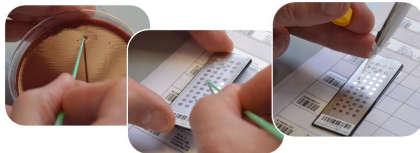
Figure 3. Preparation for colony typing on an MALDI TOF mass spectrometer.
