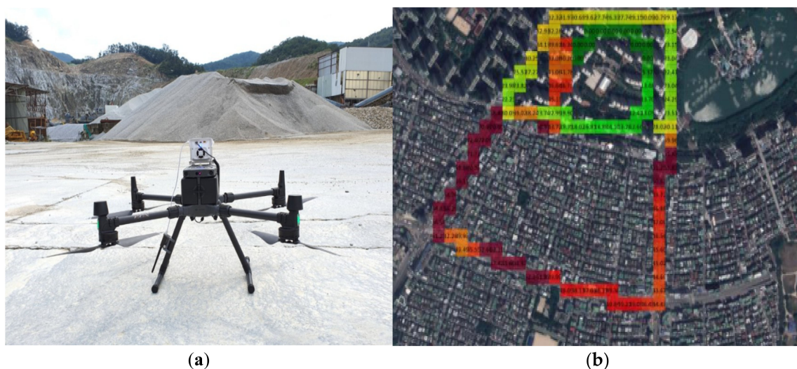
Figure 2. Measurement of the fine particulate matter (PM) concentration using a Sniffer4D module. (a) UAV with sniffer 4D; (b) 2D maps for data analyzed in Sniffer4D mapper.
