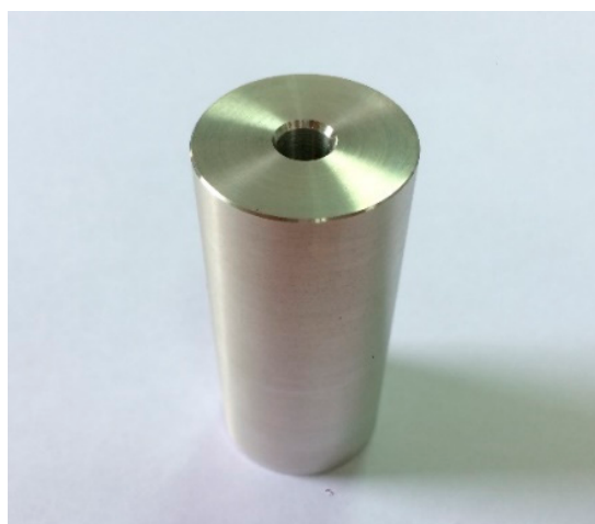
Figure 6. Photograph of the aluminium part used as a case study for the beam hardening correction; the nominal outer diameter is 25 mm, and the nominal inner diameter is 6 mm.
