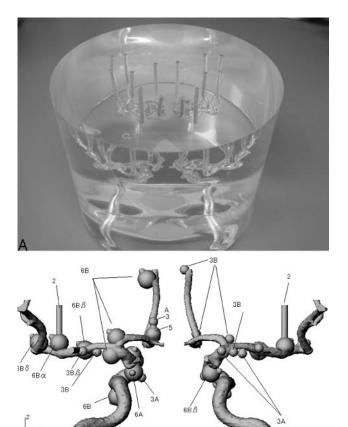
Fig 1. Photograph (A) and schematic drawing (B) of the anthropomorphic vascular phantom used in this study. The phantom was designed to simulate the intracranial arteries with a total of 32 aneurysms. Of 32 aneurysms, 15 had an aneurysmal bleb with diameter of 2 mm.
