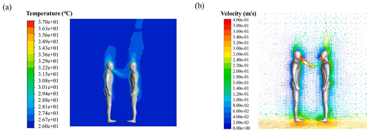
Fig. 5. The temperature distribution (a) and the velocity distribution including thermal plume (b) around the human bodies at  $Q = 30 \text{ L/min}$ .
