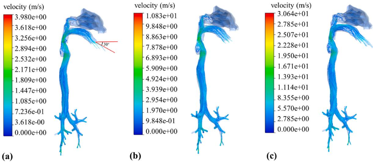
Fig. 2. Velocity streamlines in the infected individual's respiratory tract. (a)  $Q = 10$  L/min; (b)  $Q = 30$  L/min; (c)  $Q = 90$  L/min.
