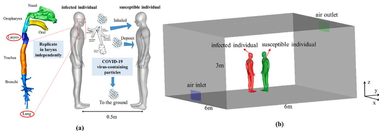
**Fig. 1.** The computational model. (a) Respiratory tract model and the schematic diagram of transmission of COVID-19 virus-containing particles (b) A typical indoor environment with a dimension of 6 m\*6 m\*3 m (L\*W\*H), and there are two breathing humans with a distance of 0.5 m, face to face.
