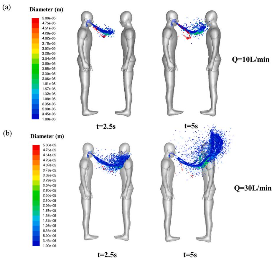
Fig. 6. The virus-containing particles' trajectories when released from larynx: (a)  $Q = 10 \text{ L/min}$ ; (b)  $Q = 30 \text{ L/min}$ .
