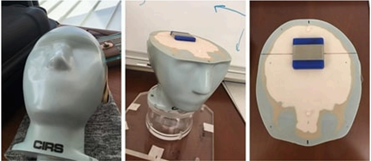
Figure 3: Photo of the customized pediatric head phantom with tissue-equivalent insert and blue bolus wax spacers used for testing the detection of anatomical changes. In these photos, the insert and spacers are oriented for an AP radiograph. The insert and spacers would be rotated 90 degrees for a lateral radiograph.
