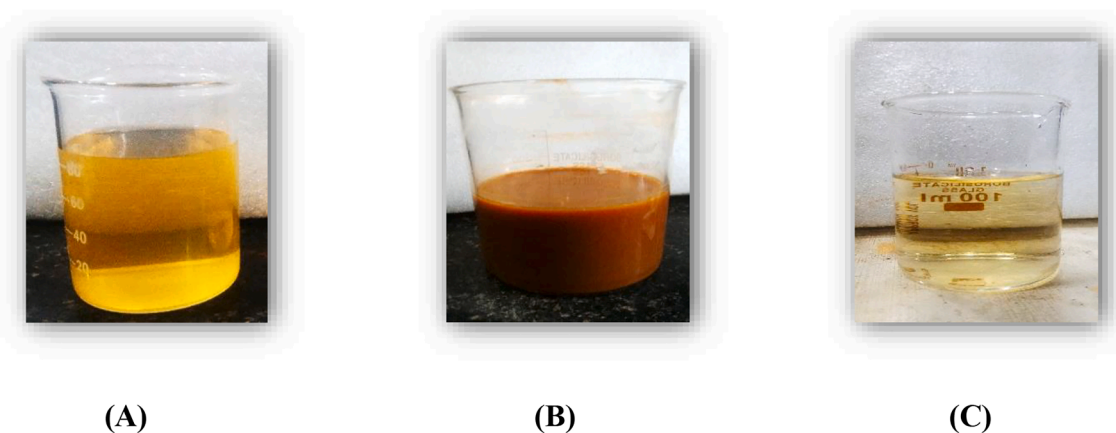
Fig. 11. Photographic representation of (A) fresh effluent-II (B) effluent-II after US + Fenton ( \text{H}_2\text{O}_2 :17.5 g/L, \text{H}_2\text{O}_2/\text{Fe}^{2+} :3) treatment (C) effluent-II after CaO (dose: 1 g/L) treatment subsequent to US + Fenton.
