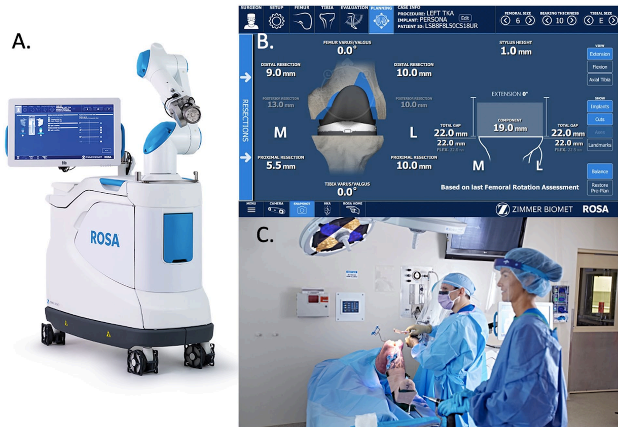
Fig. 3 (A) ROSA for total knee arthroplasty. (B) ROSA's computer software for preoperative and intraoperative planning based on implant positioning and soft tissue tensioning. (C) ROSA arm attaching cutting block for femoral cut.
