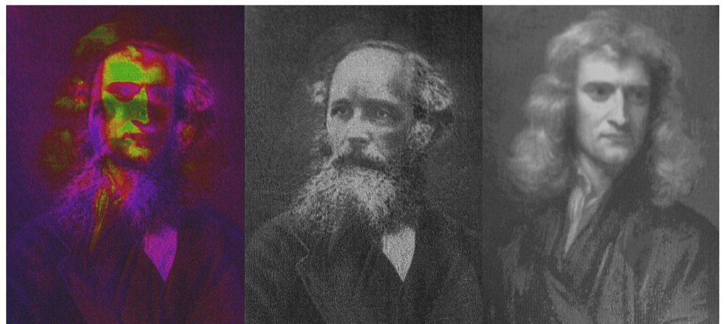
Figure 6. An image depicting encoding of information using type II modification induced birefringence. While both of the images seem to be written in the same volume (image on the left) images of Maxwell (center) and Newton (right) can be separated by exploiting imaging along both optical axes. Taken from [100].
