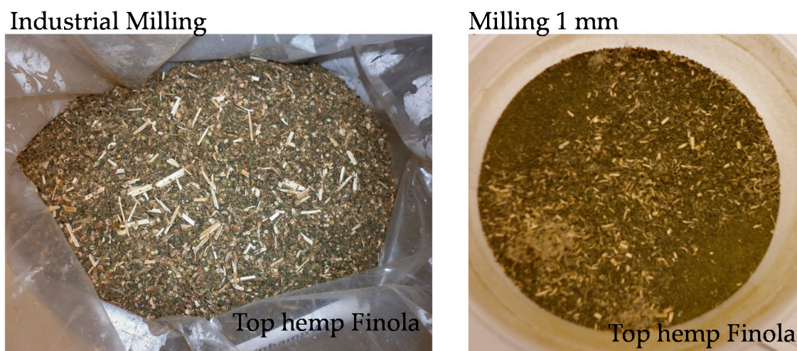
Figure 7. Examples of milled hemp. Top hemp, Cannabis sativa L. variety Finola was milled by means of industrial milling and subsequently further milled to pass through a 1-mm screen and homogenized.
