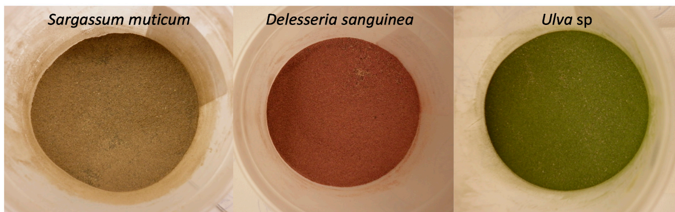
Figure 6. Examples of milled seaweeds. Brown: Sargassum muticum , red: Delesseria sanguinea and green: Ulva sp. seaweeds were milled to pass through a 1-mm screen and homogenized.
