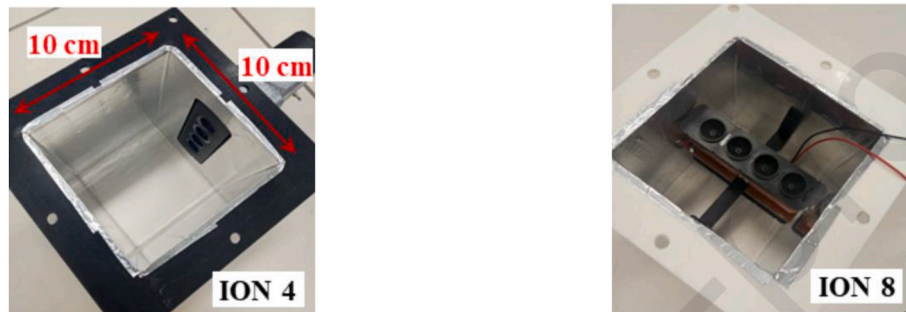
Fig. 20. Ionizers of four (ION4) or eight (ION8) corona needles (Oluwatoyin Sunday and Sakugaw, 2020).
