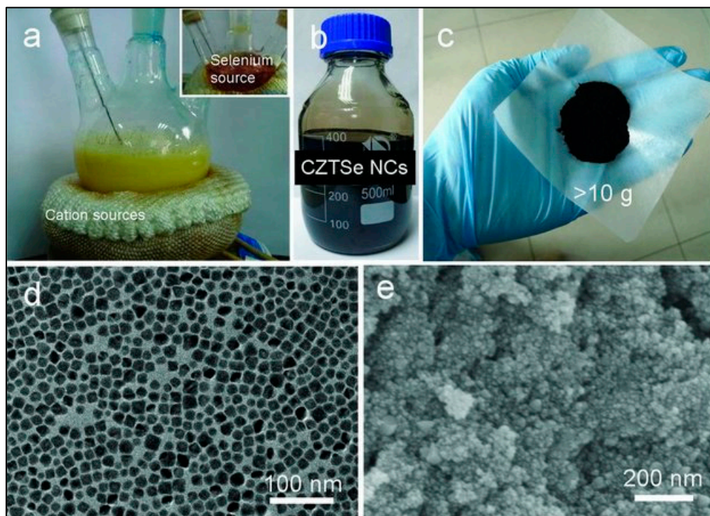
Figure 2. (a) Large-scale colloidal synthesis of copper zinc tin selenide (CZTSe) (pictures of the reaction flasks), (b) The synthesized non-stoichiometric CZTSe nanocrystals dissolved in hexane, (c) More than 10 g synthesized surface-clean CZTS nanoparticles, (d,e) Transmission Electron Microscopy (TEM) and Scanning Electron Microscopy (SEM) images of the synthesized nanoparticles. Reproduced with permission from [52]. Copyright Wiley Online Library, 2017.
