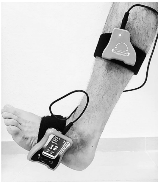
Fig. 3 Measurement of ankle proprioception by digital dual inclinometer
