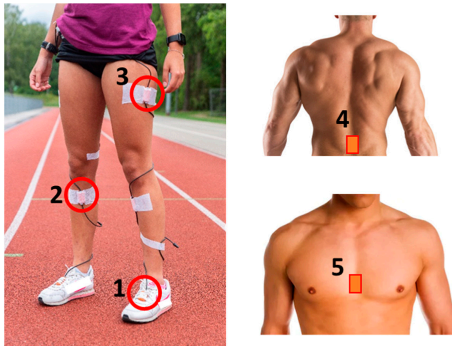
Figure 2. Measurement setup. IMUs are placed at both feet (1, highlighted left foot), both tibias (2, highlighted right tibia), both thighs (3, highlighted left thigh), pelvis (4) and sternum (5).
