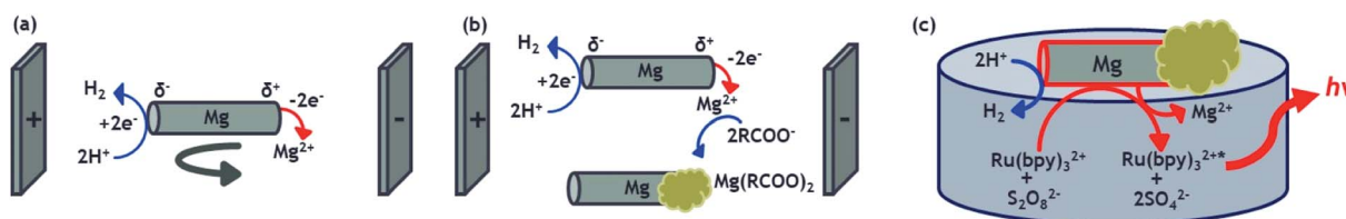
Scheme 1 (a) Illustration of the bipolar electrochemical milling process, (b) mechanism of the indirect bipolar electrodeposition of anodic electrophoretic paint and (c) motion and light emission principle of a self-propelled CL microswimmer.
