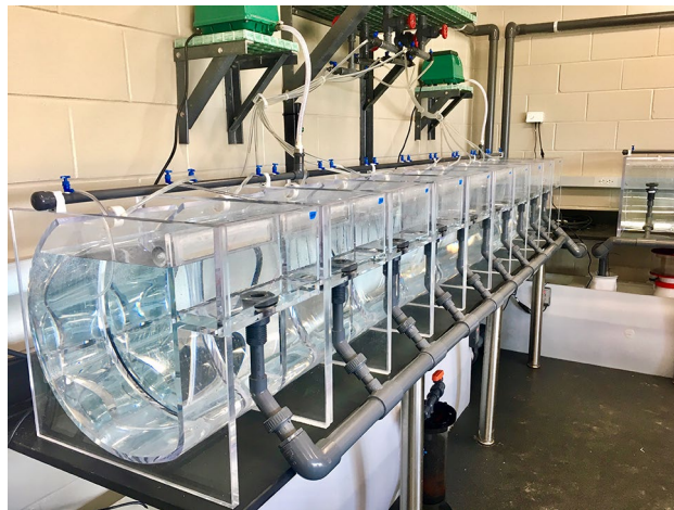
Figure 2. Photograph depicting configuration of the 1800-L recirculating larviculture system used to rear D. antillarum larvae.
