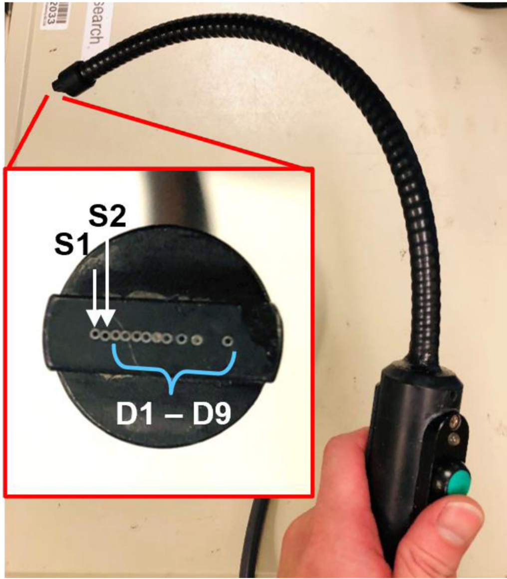
Figure 1. Image of surface contact probe of the fluorescence spectroscopy system and a close-up view of the optical fibers arrangements at the contact end of the probe. S1 and S2 are the source fibers. D1-D9 are the detection fibers.
