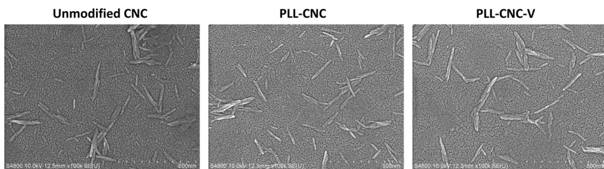
Figure 2. FE-SEM images of unmodified CNC NPs, PLL-coated CNC (PLL-CNC) NPs, and vemurafenib-loaded CNC (PLL-CNC-V) NPs, scale bar = 500 nm.
