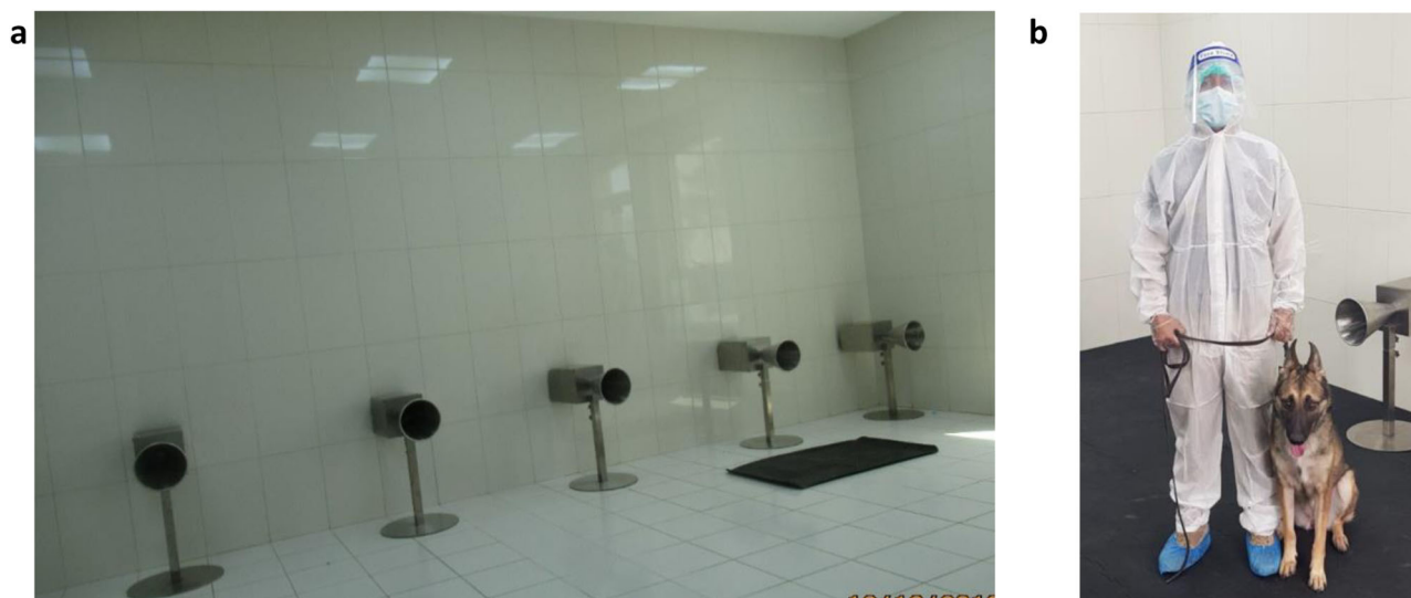
Fig. 2 Training stations lined up at the Federal Customs Authority (FCA) facilities in Abu Dhabi, United Arab Emirates, for the training of explosives detection dogs. a Training devices with samples' containers placed right behind the metal olfaction cones. b The dog handler is deployed to work with the dog as a team.
