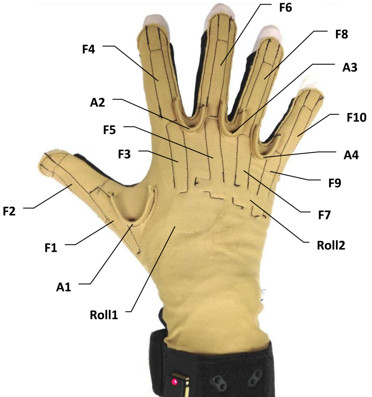
Fig. 1. 18-sensor Cyberglove sensor location (the two sensors related to the wrist are not sketched as they are not used)
